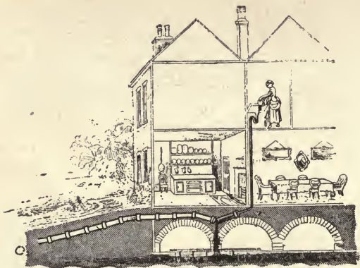
Fig. 637. Cellar kept damp twelve years by slopwater.
